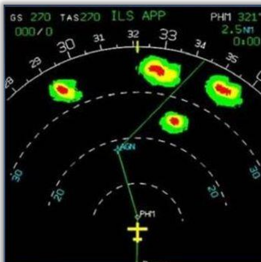
Figure 13 – Cockpit weather display showing four strong cells 25-35 miles ahead of the aircraft.
