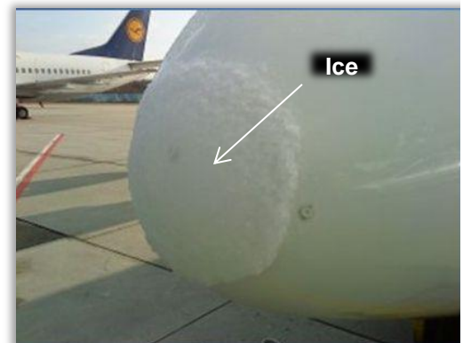
Figure 10 – Ice buildup on an aircraft’s radome.
