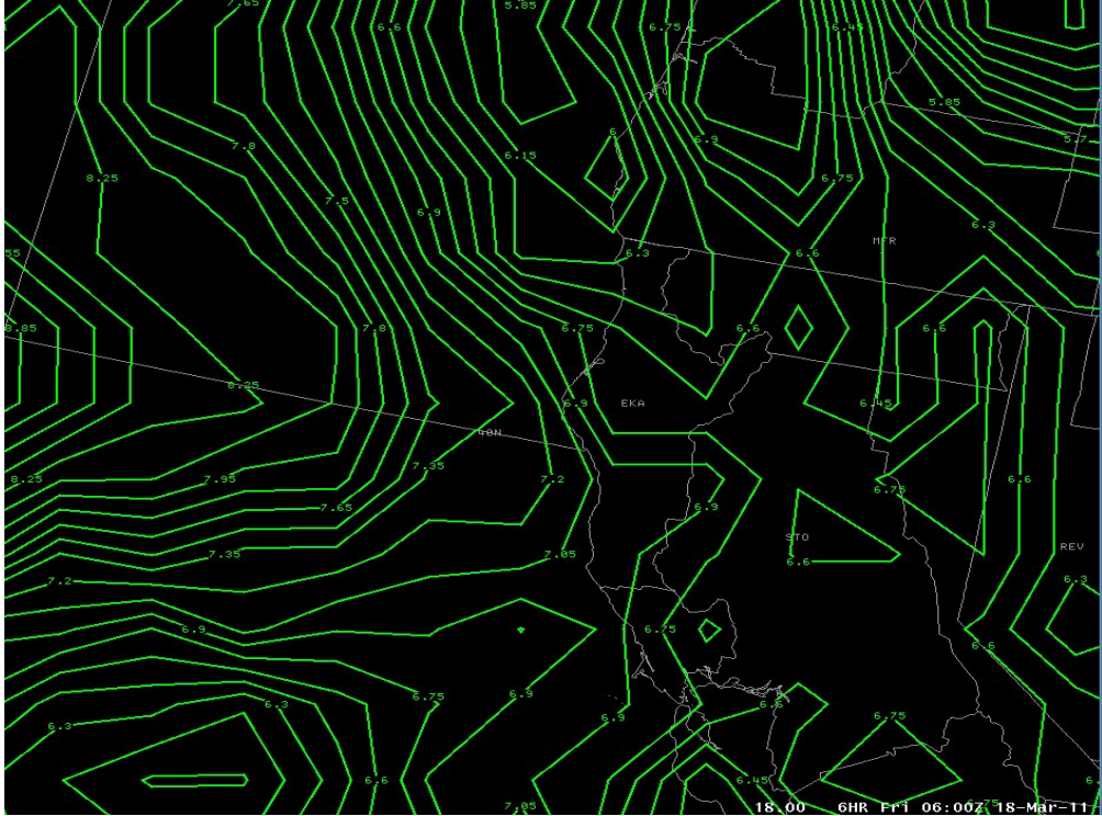
Figure 5: 925 to 850 MB lapse rates of 6 to 8 degrees C/km showing general instability.
