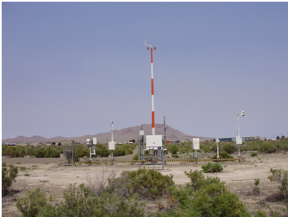
The Automated Surface Observing System (ASOS) at the Winnemucca Municipal Airport currently produces the official weather observations for Winnemucca. Photo by author.
