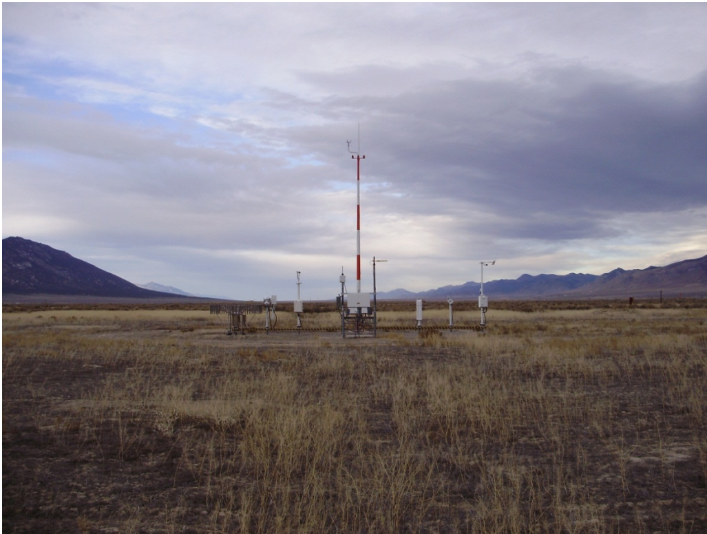
The Automated Surface Observing System (ASOS) at the White Pine County Airport currently produces the official weather observations for Ely.
