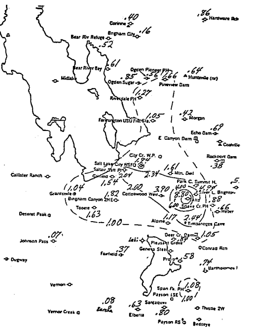
Figure 15 - Total water equivalent precipitation for all Lake cases in which the average 700 mb wind direction was from 300 to 310 degrees (inclusive).
