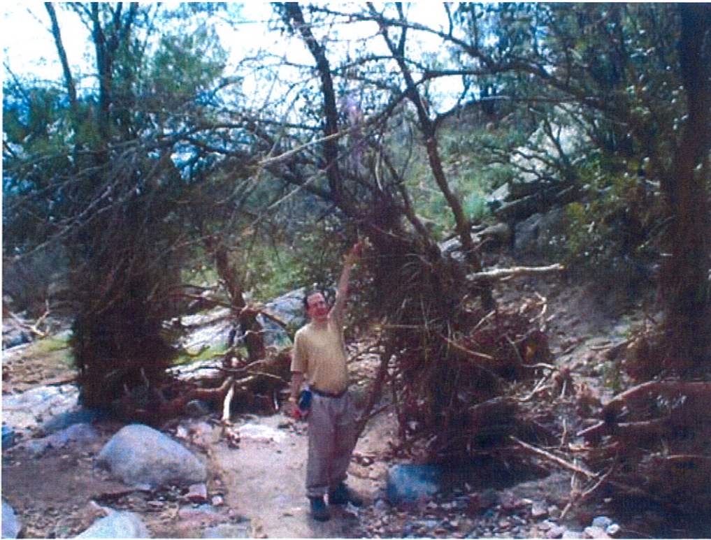
Figure 9. NWS hydrologist Mike Schaffner pointing out a debris line in a tree located in the upper slope-area reach.
