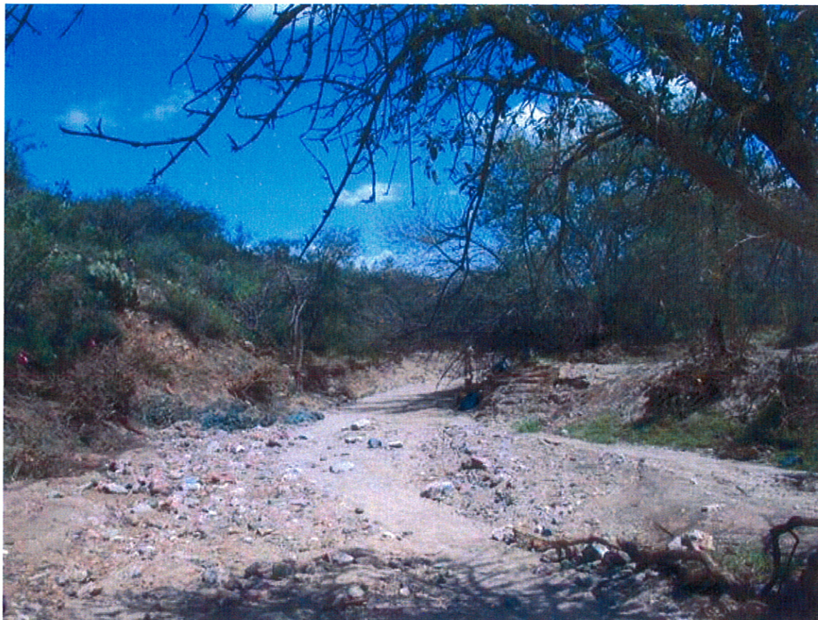
Figure 10. Image of lower slope-area reach looking downstream. Notice pink flagging on left bank indicating high water marks to be surveyed in. Photo courtesy of USGS.
