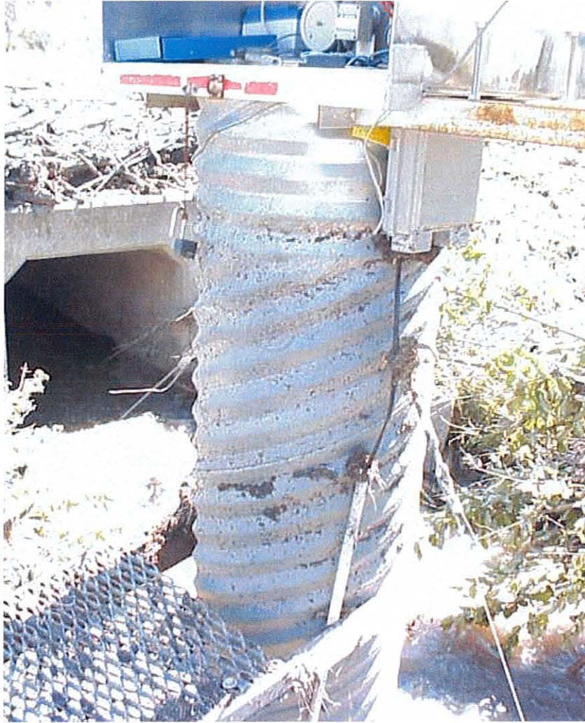
Figure 3. USGS river gage and tipping bucket precipitation gage with recording devices at mouth of Laird Creek.
