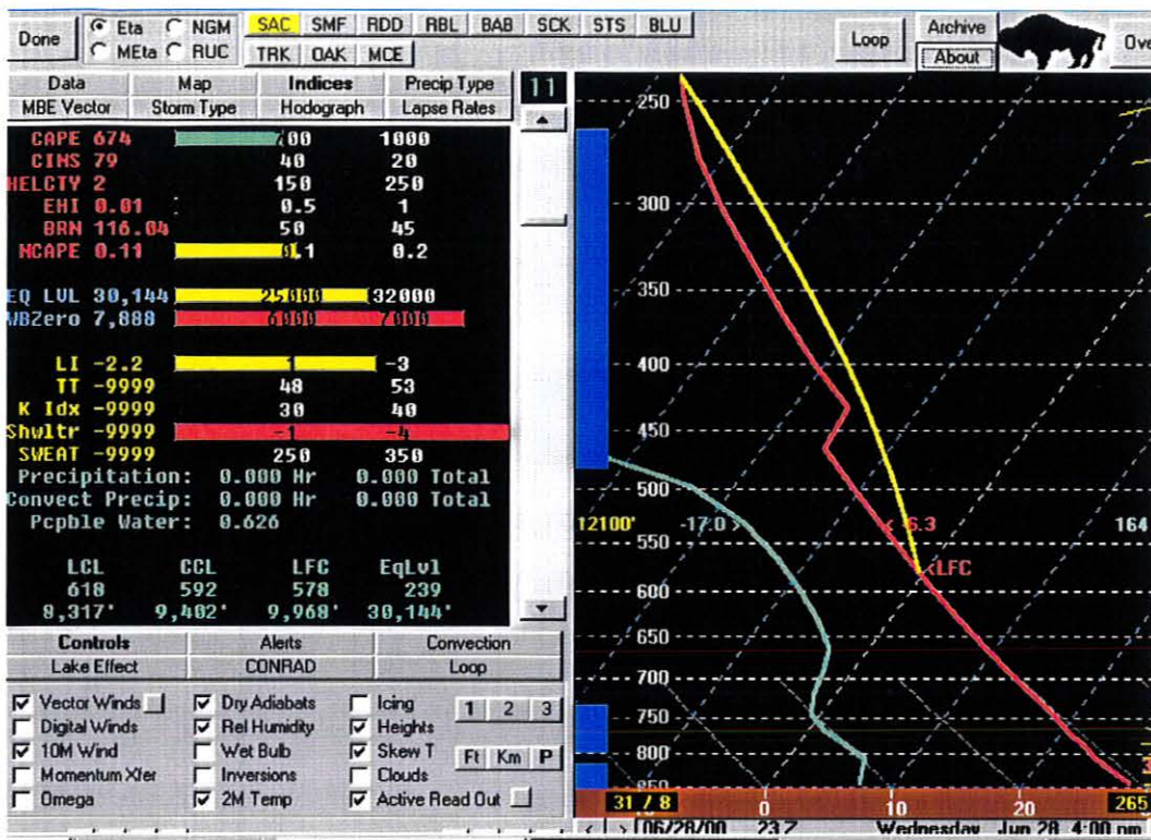
Figure 19. A BUFKIT Eta profile at 2300 28 June 2000 from the 1200 UTC 28 June run. The NCAPE value was 0.11 \text{ ms}^{-1} .
