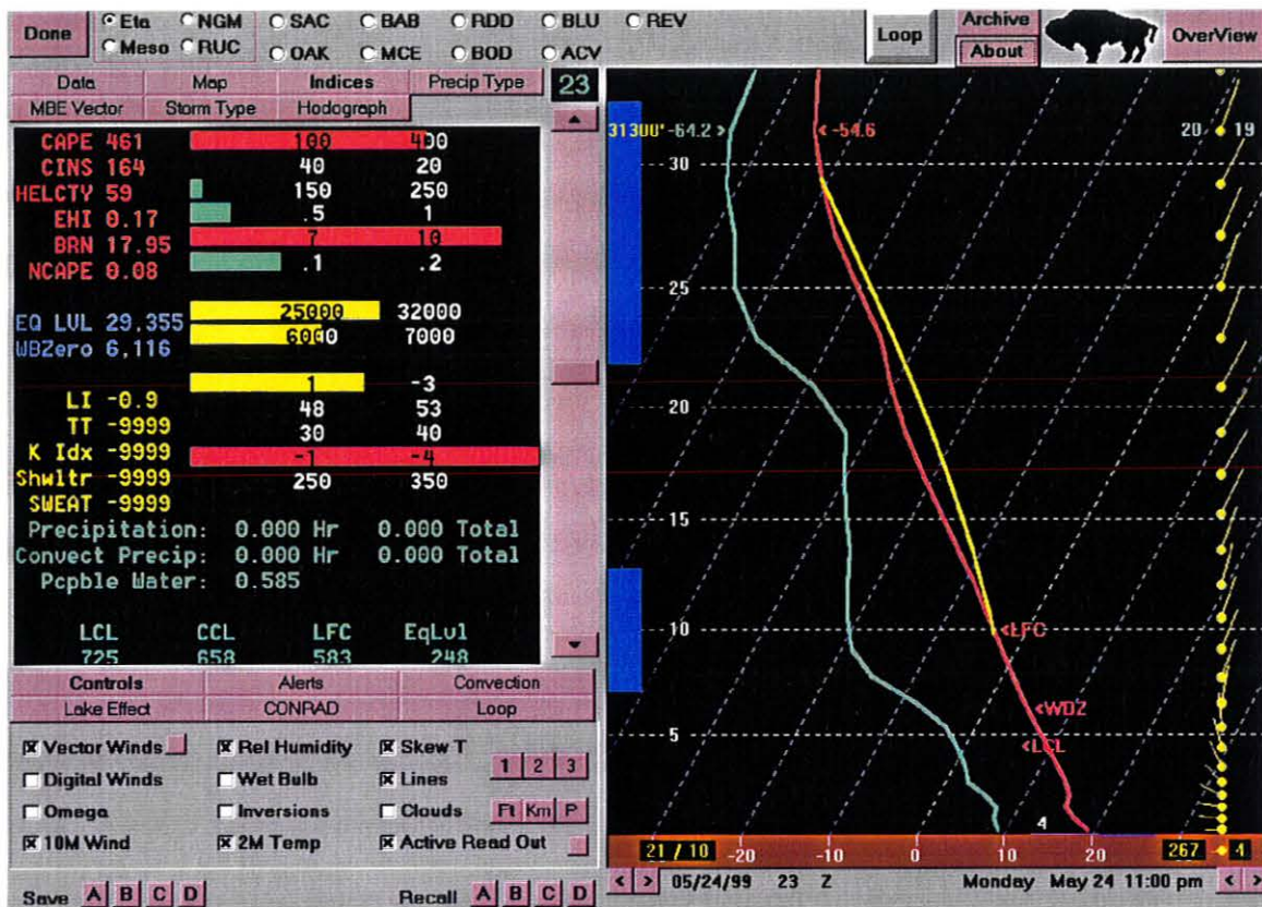
Figure 3. KBLU sounding displayed in BUFKIT at 2300 UTC on 24 May 1999 from the 0000 UTC Eta model run 24 May. The yellow line on the sounding clearly shows the large area of forecast instability (CAPE) with an equilibrium level at 30-kft. The table on the left shows various forecast parameters including CAPE, NCAPE, and LI.
