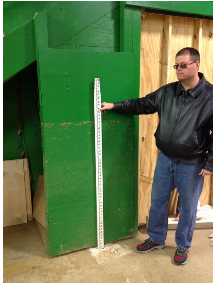
Fig. 23. Lee Creek high water mark inside the Field of Dreams baseball complex indoor batting practice facility in Van Buren. (Image: Nicole McGavock, NWS Tulsa; Michael Lacy pictured)
