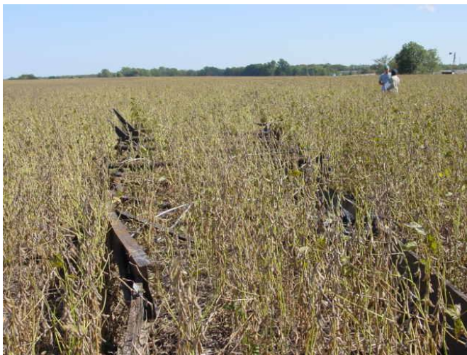
(Tornado #2) Remains of the base frame from the single wide mobile home. The base frame was tossed by the tornado and located a third of a mile to the north-northwest of the mobile home's initial site in a soybean field. Debris from the tornado (e.g. clothing, pieces of furniture) was displaced as far as 3 to 4 miles to the north of the initial mobile home site (Viewing north-northwest).
