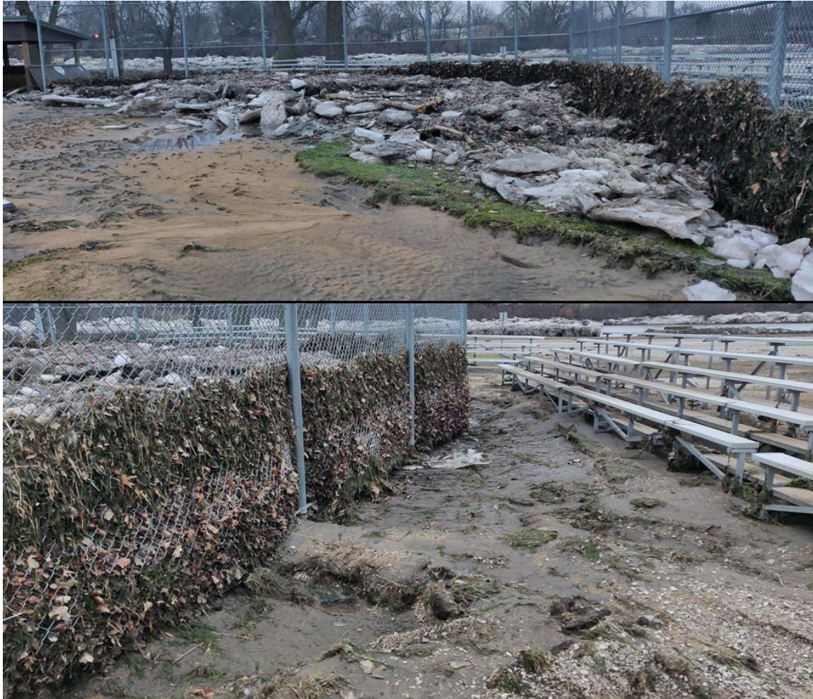
Figure 16. Vegetation stuck in the fence at baseball field at North Island Park (downstream end) in Wilmington. These high water marks suggest a peak water level of about 536 feet elevation. Photographed on January 30.
