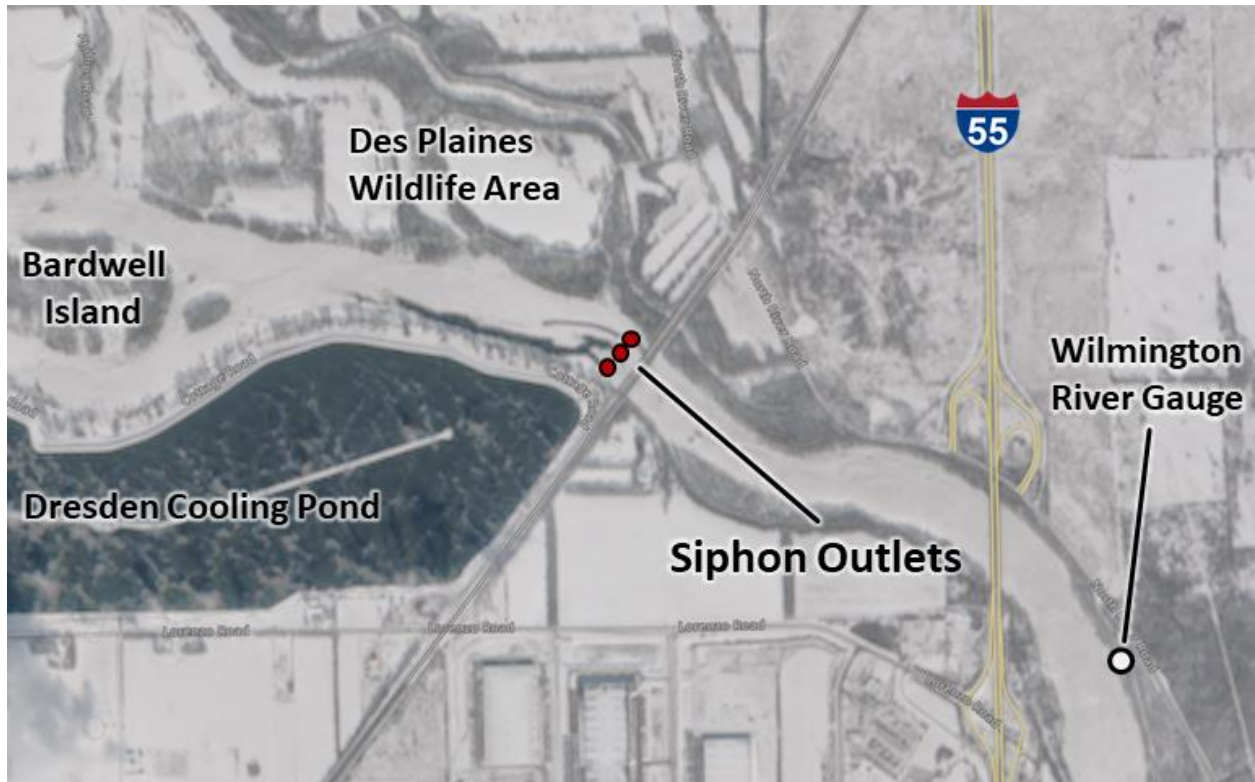
Figure 6. Aerial imagery of the lower end of the ice jam on January 20, 2024, captured by the Sentinel2 satellite. Paths of melting ice due to operation of the warm water siphon system are visible extending from near the railroad bridge downstream toward Bardwell Island. Imagery courtesy of Copernicus Sentinel data.
