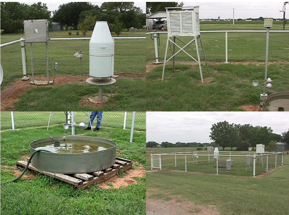
COOP Station including temperature, precipitation, and evaporation equipment.
