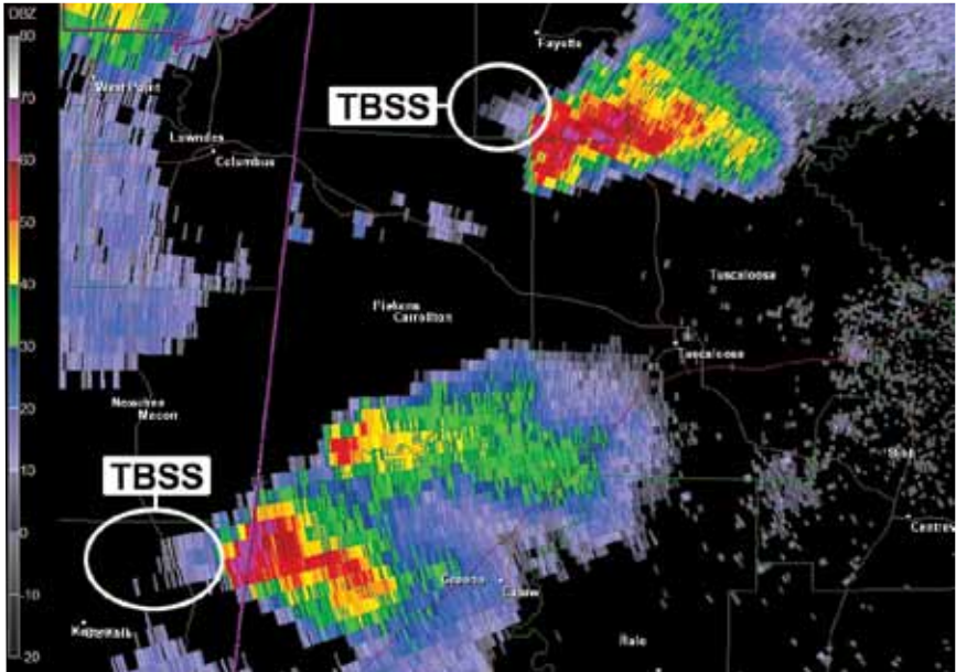
Three Body Scatter Spike on June 6, 2005, Cannon Air Force Base, NM, radar.
