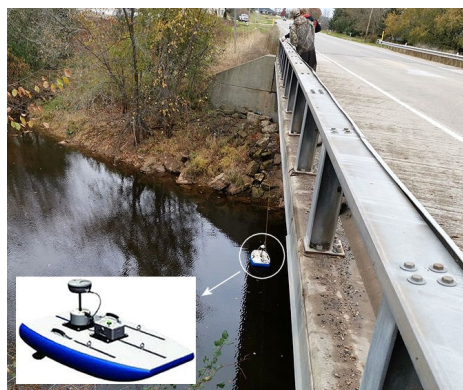
Figure 4: Surveyor unit measures the bathymetry and discharge.
