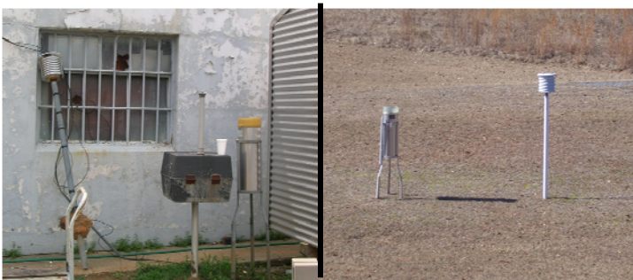
An extreme example of improper sensor siting due to construction at an observation site (left), and the improved siting made by our staff on a grassy, open area (right).
