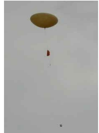
Balloon, parachute and radiosonde in flight.
