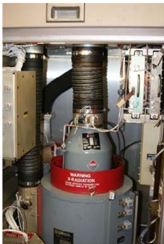
Klystron used to amplify WSR-88D radar power from milliwatts up to one megawatt.
