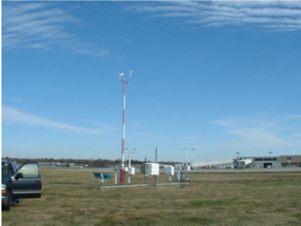
Figure 16. The Automated Surface Observing System at the Des Moines, Iowa, airport as of 2005. View is looking northeast.
