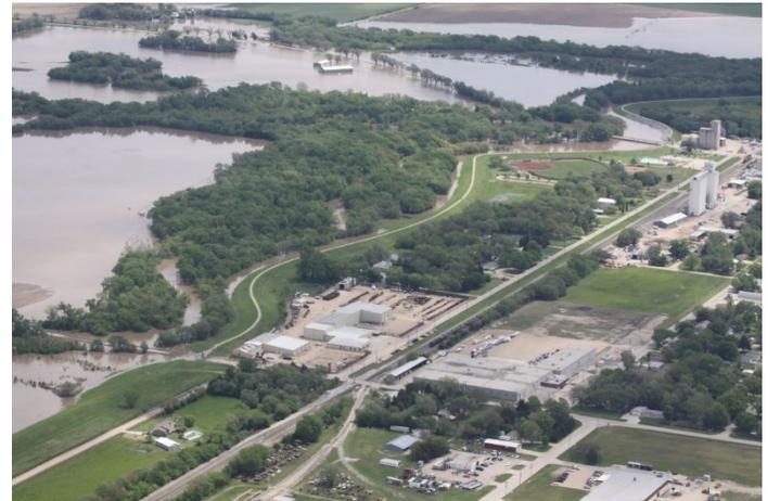
**Figure 5: A levee system around the town of Halstead holds back the swollen Little Arkansas River in May.**
