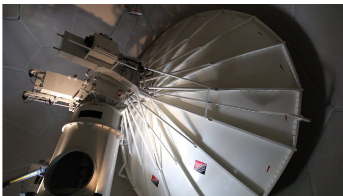
The radar receiving dish inside the protective cover. Dual-pol is both a hardware and software upgrade to the radar.
